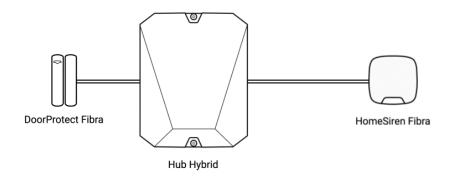
DoorProtect Fibra is a wired opening detector. The detector is connected to the hub via a wired bus and operates using the Fibra protocol. In case of standard installation, it consists of two blocks: a detector and a magnet. The detector is mounted on a frame or fixed part of the structure, and the magnet is mounted on a movable flap or a sliding part.
